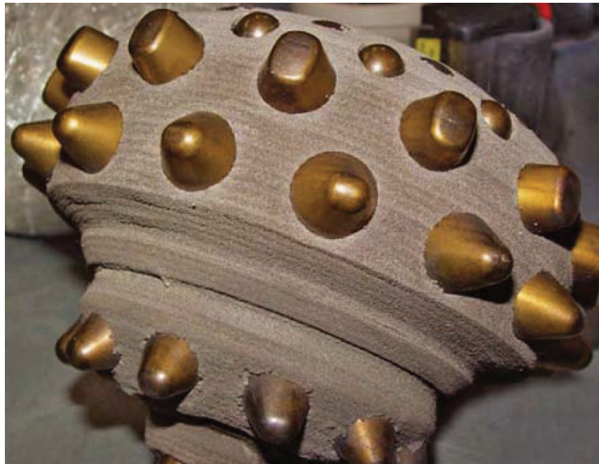
Sample of cladding of dissimilar metals on a downhole drill bit. This photo illustrates laser cladding being used to protect critical component wear surfaces and extend service lives. A similar process was used for the NASA-SSC project. Photo courtesy of Laser Cladding Services Ltd.
