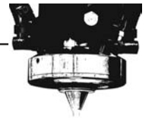
LCS has applied tungsten carbide hardfacing via the laser cladding process in order to protect these tools in downhole service. Photo courtesy of Laser Cladding Services Ltd.
