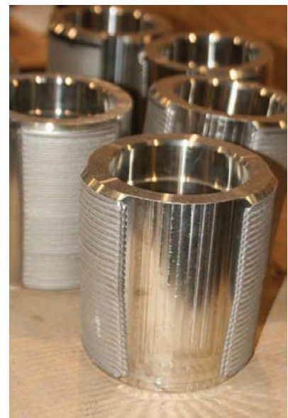
Shown are tools used in a downhole drilling application that have been coated horizontally on a raised portion of the circumference with a tungsten carbide-based hardfacing. Photo courtesy of Laser Cladding Services Ltd.
