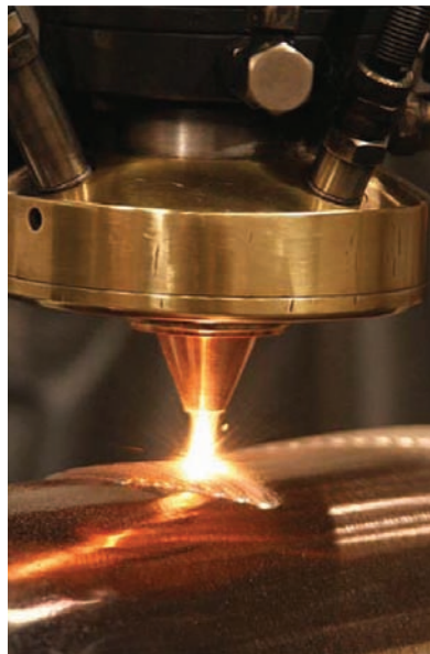
Laser Cladding Services' proprietary laser technology bonds a metallic powder, which is blown through the brass nozzle at the laser's base and intersects with the beam and metal being clad. The result is a bead of metal that is metallurgically bonded to the object. Photo courtesy of Laser Cladding Services Ltd.
